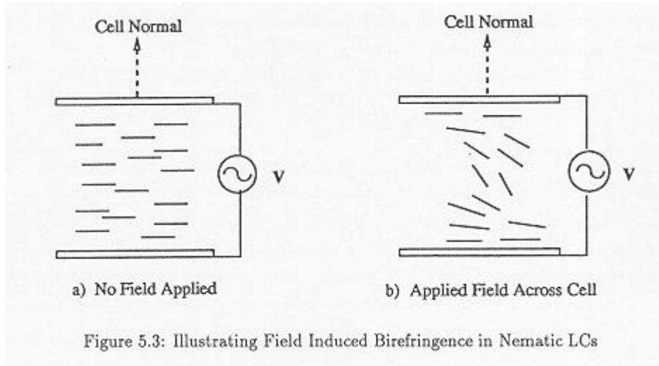
Figure 5.3: Illustrating Field Induced Birefringence in Nematic LCs
