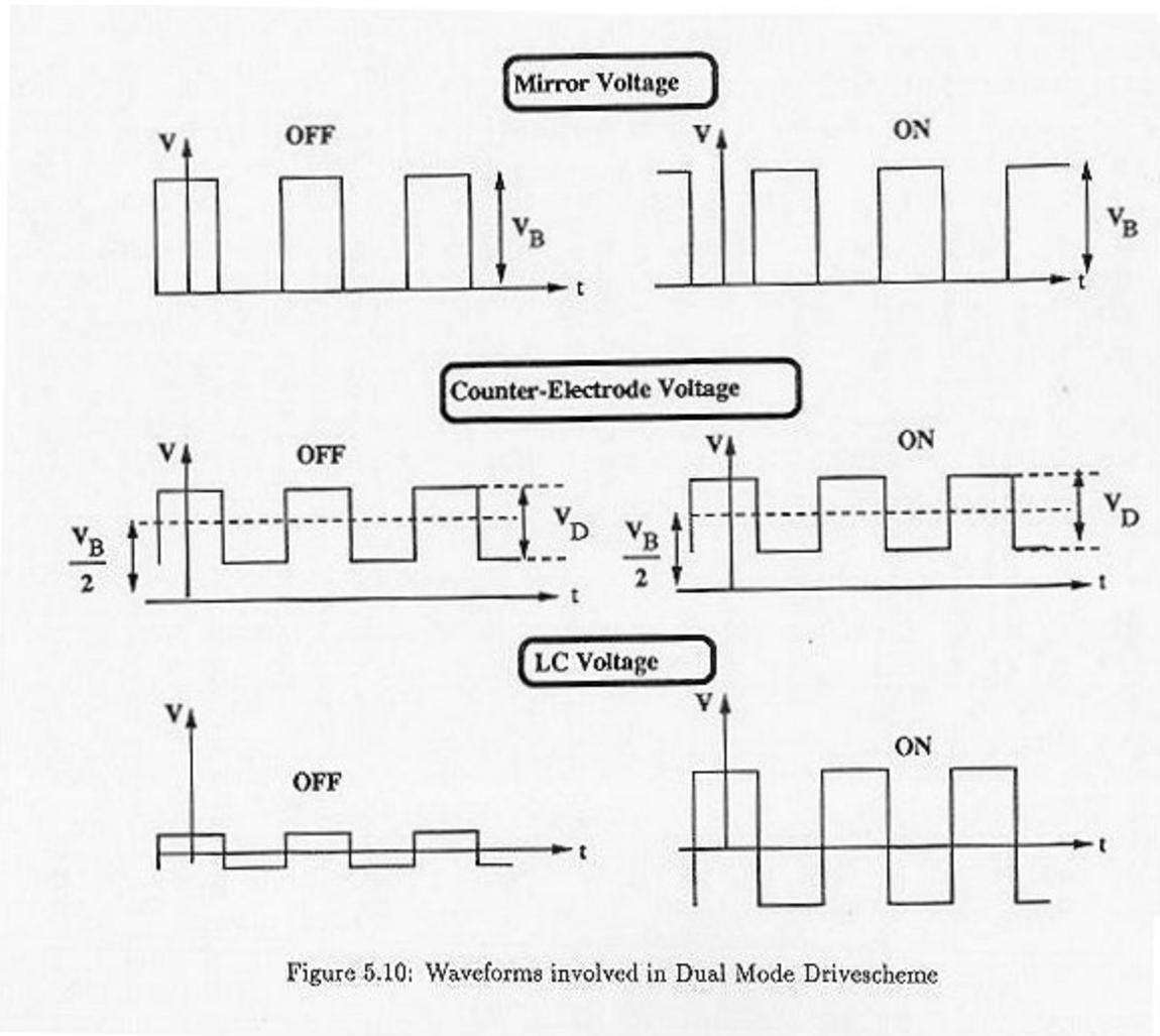
Figure 5.10: Waveforms involved in Dual Mode Drivescheme
