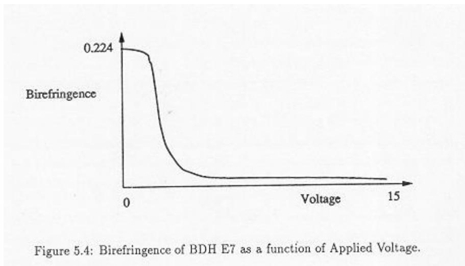
Figure 5.4: Birefringence of BDH E7 as a function of Applied Voltage.
