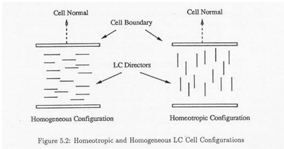
Figure 5.2: Homeotropic and Homogeneous LC Cell Configurations
