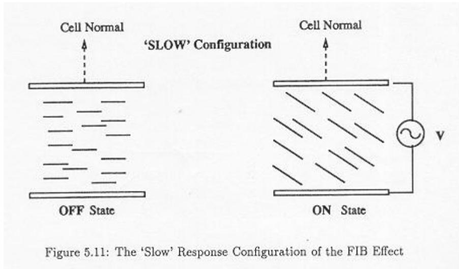
Figure 5.11: The 'Slow' Response Configuration of the FIB Effect
