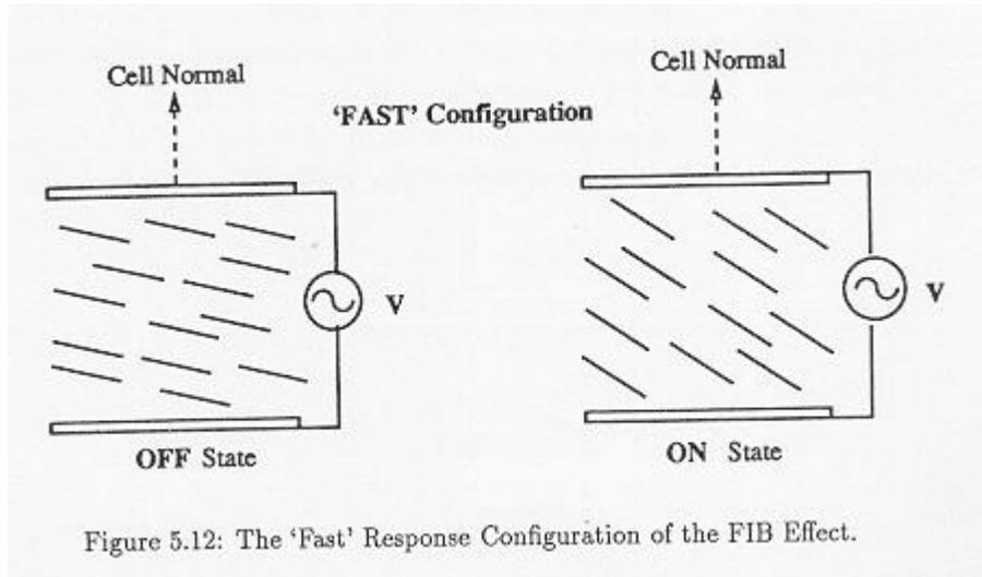
Figure 5.12: The 'Fast' Response Configuration of the FIB Effect.
