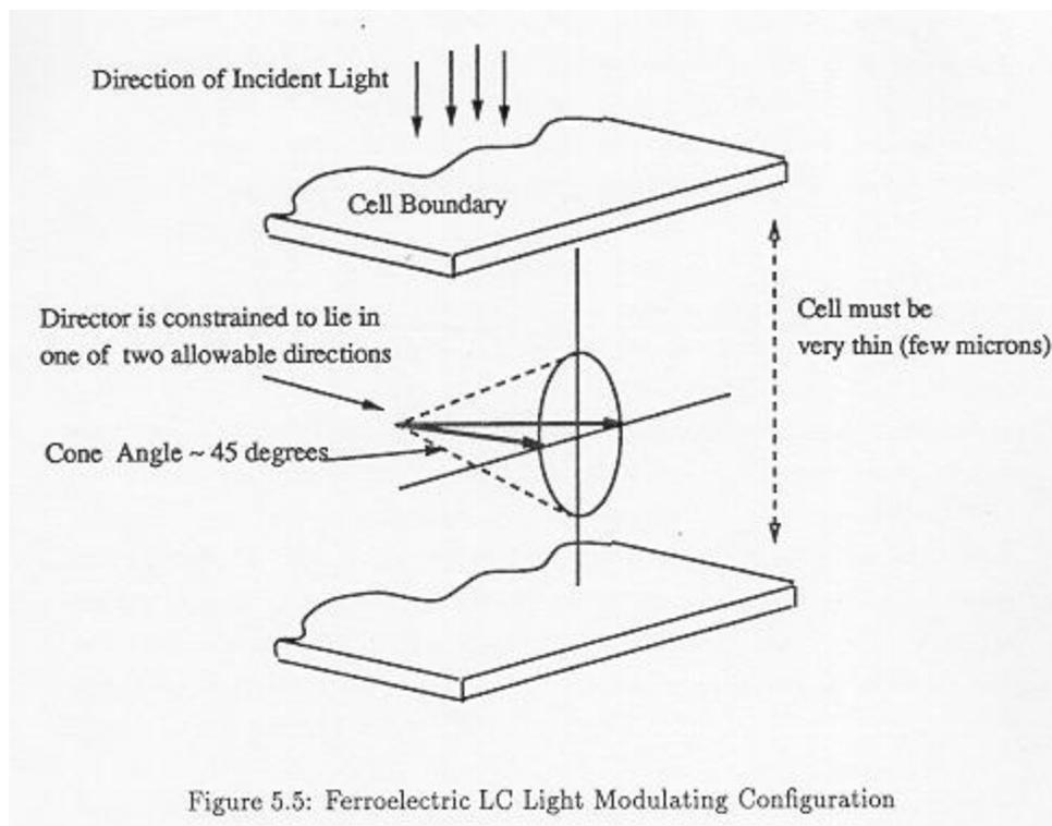
Figure 5.5: Ferroelectric LC Light Modulating Configuration
