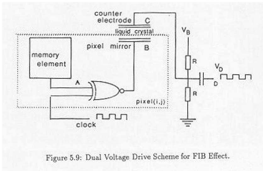
Figure 5.9: Dual Voltage Drive Scheme for FIB Effect.
