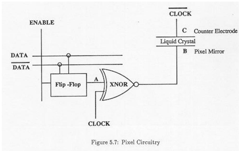
Figure 5.7: Pixel Circuitry
