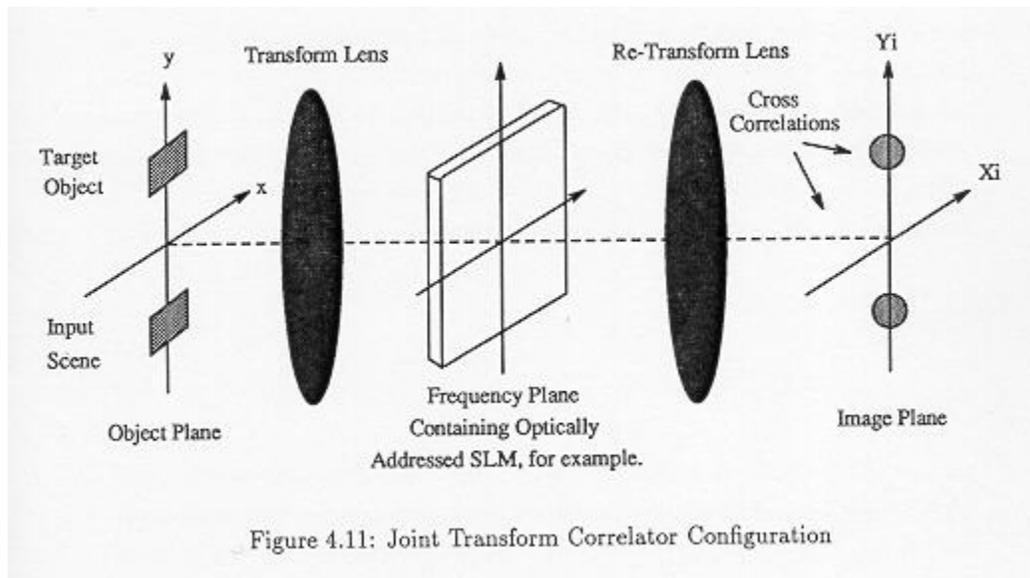
Figure 4.11: Joint Transform Correlator Configuration
