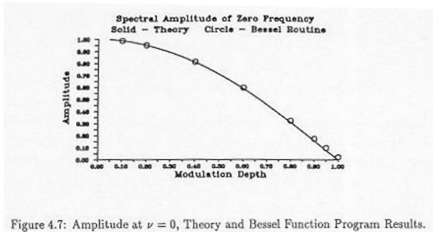
Figure 4.7: Amplitude at  $v = 0$ , Theory and Bessel Function Program Results.
