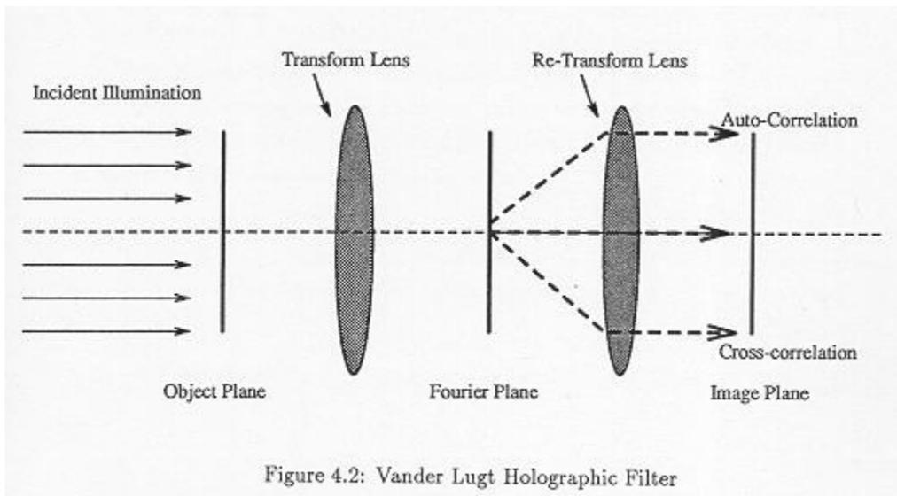
Figure 4.2: Vander Lugt Holographic Filter
