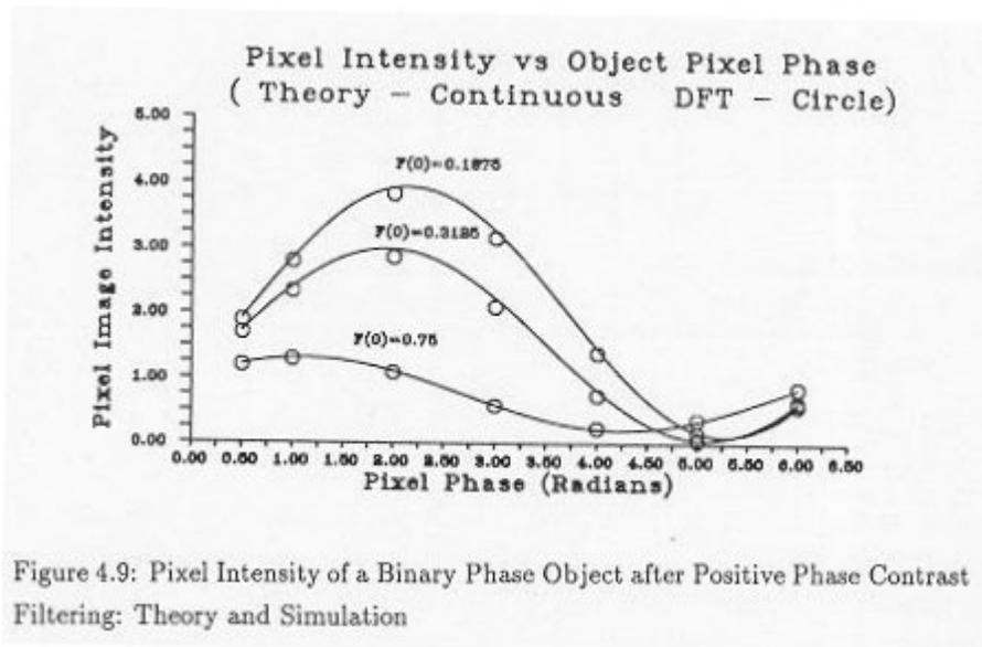
Figure 4.9: Pixel Intensity of a Binary Phase Object after Positive Phase Contrast Filtering: Theory and Simulation
