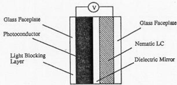
Figure 4.3: Operation of the Hughes LC Light Valve SLM
