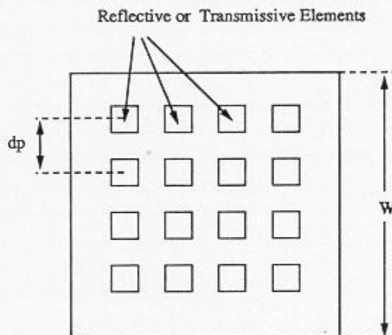
Figure 4.4: Characteristics of a Pixellated Spatial Light Modulator
