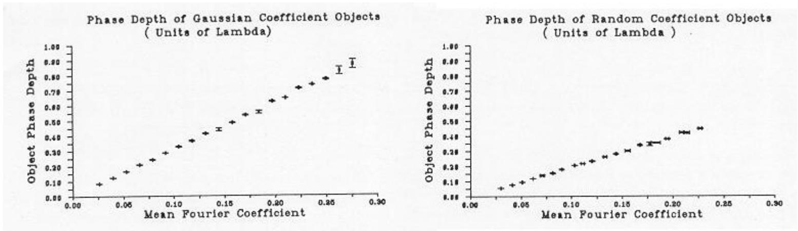
Figure 3.6: Depth of Phase Modulation: Random and Gaussian  $a_j$
