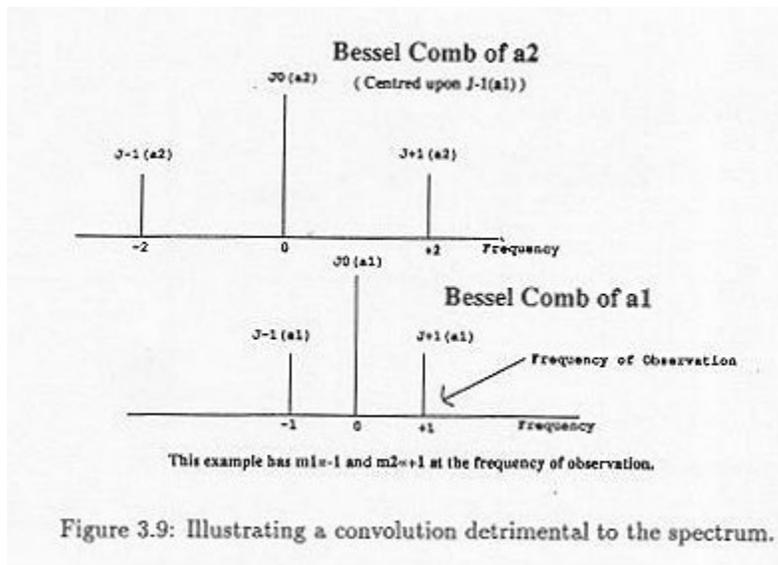
Figure 3.9: Illustrating a convolution detrimental to the spectrum.
