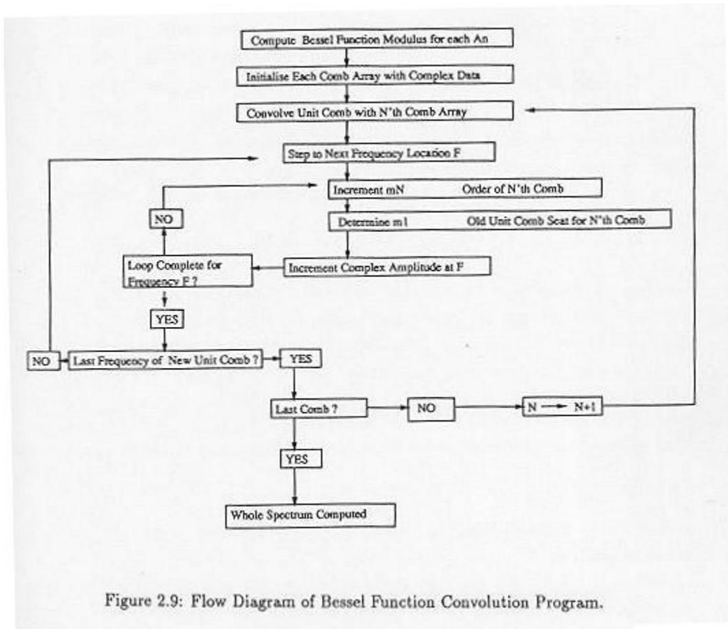
Figure 2.9: Flow Diagram of Bessel Function Convolution Program.
