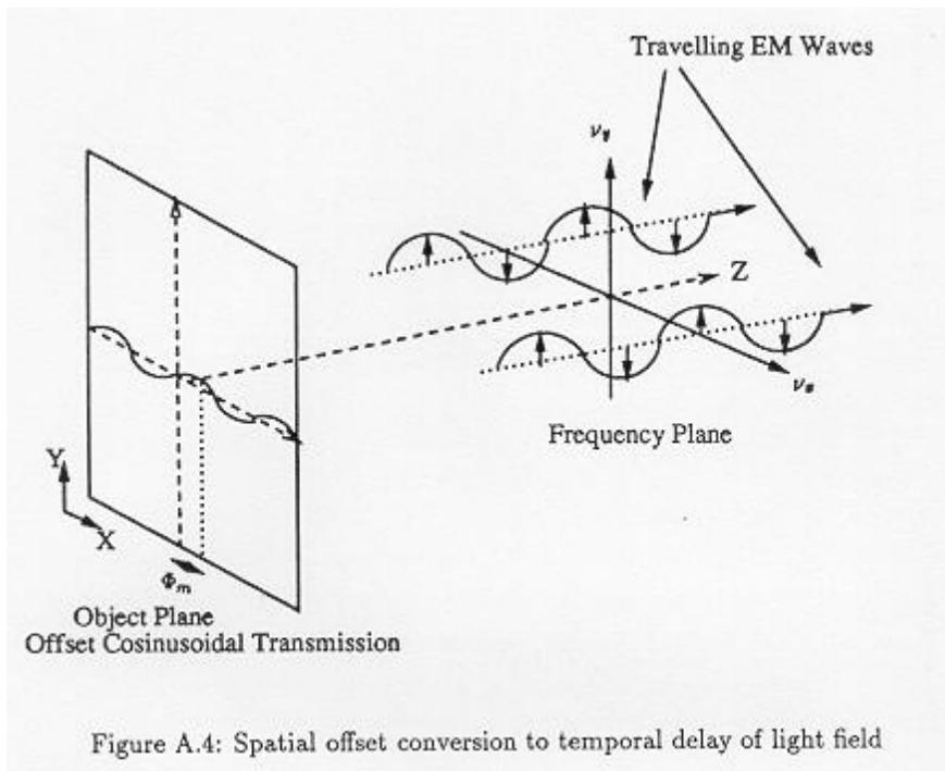
Figure A.4: Spatial offset conversion to temporal delay of light field
