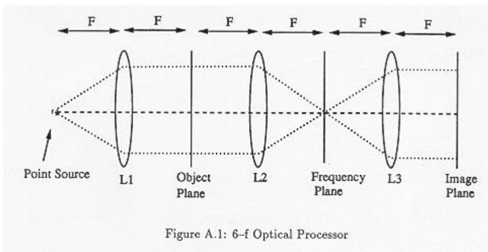
Figure A.1: 6-f Optical Processor
